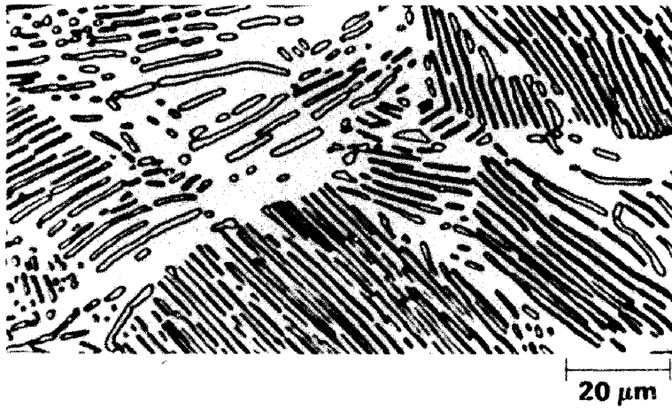
Fig. 3(d). Eutectoid steel 1080: iron carbide (dark) in ferrite matrix (light). Courtesy, ASM ( Metals Handbook , Vol. 9, 1985).
